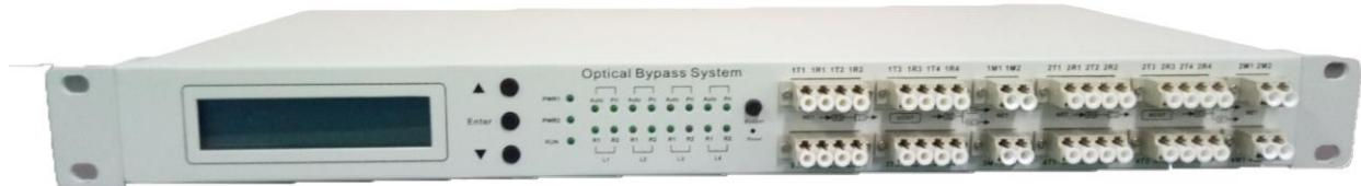
Optical bypass protection system integrates optical switching modules, optical monitoring modules and heart rate monitoring, which provides bypass protection when optical network node equipments appear power interruption, hardware failure, software deadlock etc to insure the normal signal transmission. Mainly used in flow control equipment, signal safety analysis, gigabit data communications and other fields.
