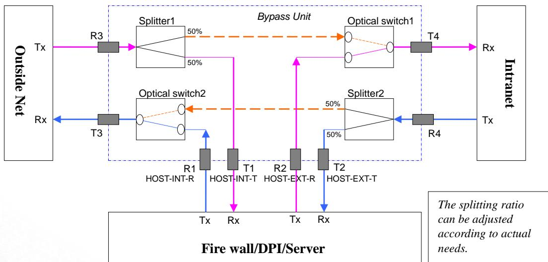
The splitting ratio can be adjusted according to actual needs.
